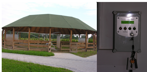
Fig. 6.14. The horse exerciser (four compartments) and its control panel (made by Consult S) 3
